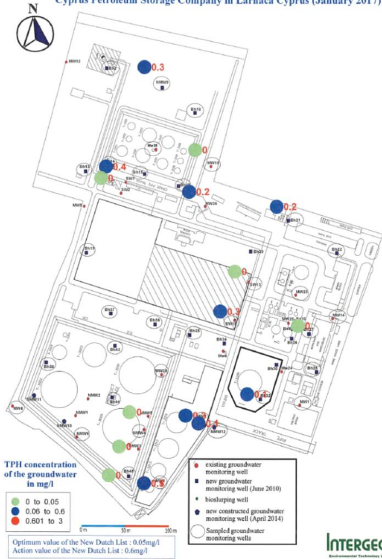
Figure 8 : Distribution of the TPH concentration of the groundwater at the area of Cyprus Petroleum Storage Company in Larnaca Cyprus (January 2017)
